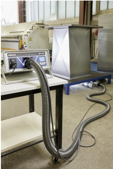
Fig. 12: Example: Measurement according to DIN EN 15727
