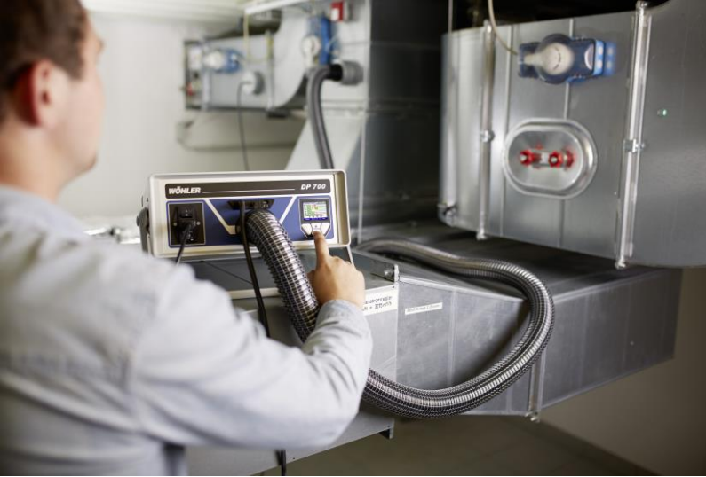
Fig. 11: Example: positive pressure measurement without adapter
