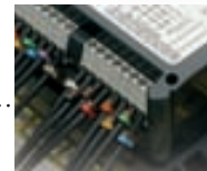
Simplified connection with screw-on terminal strip
