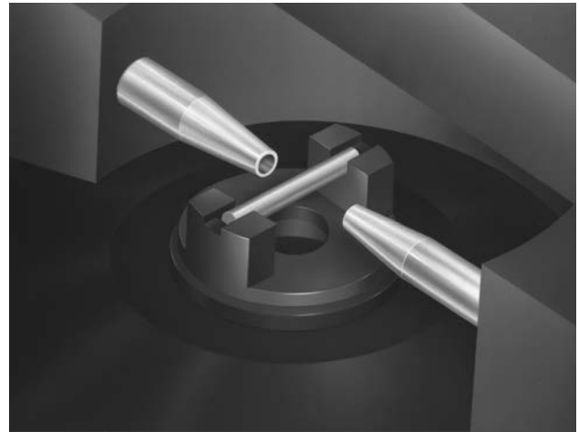
Figure 1. Detail of Deflector/Nozzle Pilot Stage
